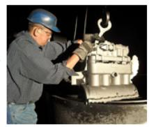
mains, rods, and camshaft, streamlined intake ports, hard exhaust seats, thicker (3/16") water jacket wall on the water inlet side, Model B water deflector, added material between exhaust ports and cylinder, replaceable cam bearings, rear main seal that is available at any bearing supply house, and many other things. The good news is that the Model A engine project has been resurrected and is now alive and well."
