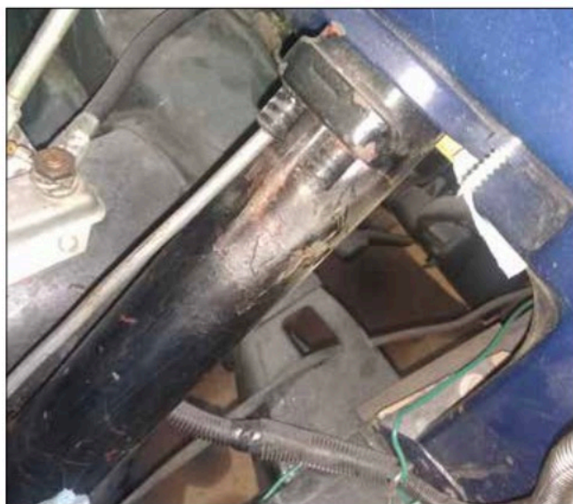
Figure 1: I put a \frac{3}{16} " rod up the steering column.
