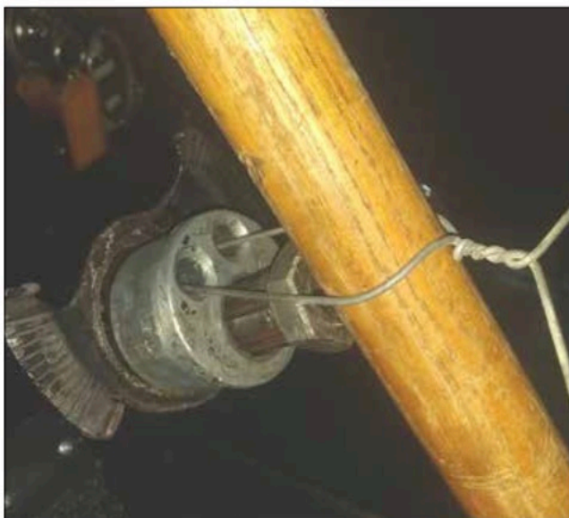
Figure 2: I threaded baling wire through the bushing and wrapped it around a section of closet rod.
